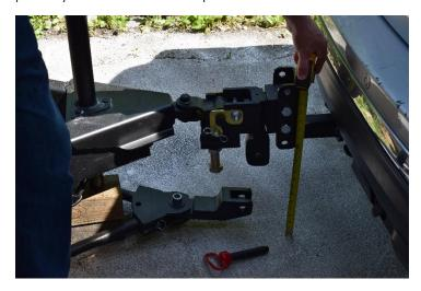
**Step 7.** Jack up the trailer AND the rear of the vehicle about 2 to 2-1/2 inches higher that the value recorded in step 4. Don't let it down until after step 17.
