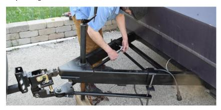
**Step 15.** Raise the jack back up and remeasure like in step 4. This value should be equal to or no more than 7/8" less than the value found in step 4.
