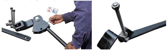
**Step 8b:** Insert the 5/8" Acme bolts through the bottom of the springs and then through the bottom of the spring tensioning brackets. Place the spherical washer with the convex side down onto the 5/8 acme bolt. Screw an acme nut onto the bolt with no more than a single thread protruding out of the top of the nut.
