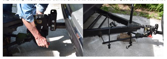
**Step 11.** Place the spring tensioning brackets on the trailer frame and screw the 1/2" bolts into the spring tensioning brackets. Don't tighten them yet. Just bring them close to the frame.
