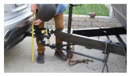
**Step 16.** Attach the safety chains for on road use and attach any break away cables and electric connections.
