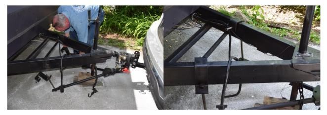
**Step 12.** Raise the spring bars up by using the 5/8" acme bolt & nuts. . Adjust the 1" angle adjustment bolt up or down to create the right distance. There should be 6-8" of gap between the springs and the bottom of the trailer frame. At this point in the procedure the 1" bolt should be tight against Item 3. NOTE: If you are compensating for a heavy load it is better to start with the larger 8" gap.
