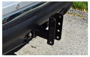
**Step 2**. With your trailer level, measure from the ground to the center of the coupling shaft. (This assumes a Lock N Roll is already installed on the trailer)
