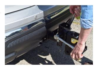
**Step 4.** Before hitching the trailer, pick a spot that is easy to measure from on the vehicle such as the center of the rear wheel well or the top of the height adjustment channel. Record the distance from the ground to your chosen point.
