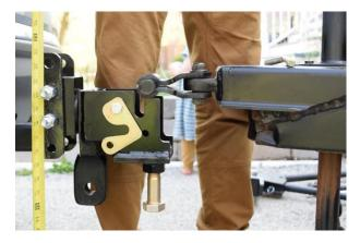
**Step 5**. Place the coupling shaft into the slots on the vehicle side and secure the latch plates with the hitch pin. Let the full weight of the trailer rest on the vehicle.
